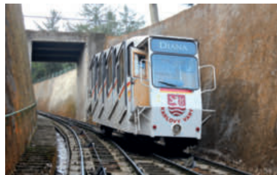
Car built in 1987 on the Abt passing loop of the Diana funicular
