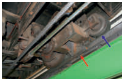
Wheelset of the Diana funicular on the side of the guiding rail on the Abt switch for car no 1. The red arrow marks the track brake and the blue arrow the flangeless wheel. The dual-flanged wheel ensures that one of the wheels of each wheelset always follows the guiding rail.
