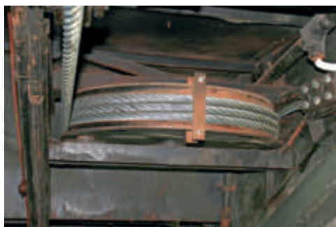
Drum for haul rope attachment to the car ( Diana funicular)
