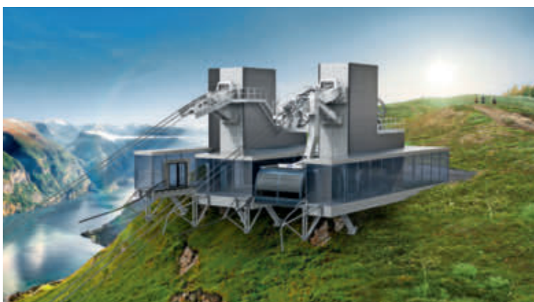
The new Peak Line station concept for reversible aerial tramways is a modular solution with clearly defined interfaces to planners, architects and civil engineers for shorter project planning and completion times.
