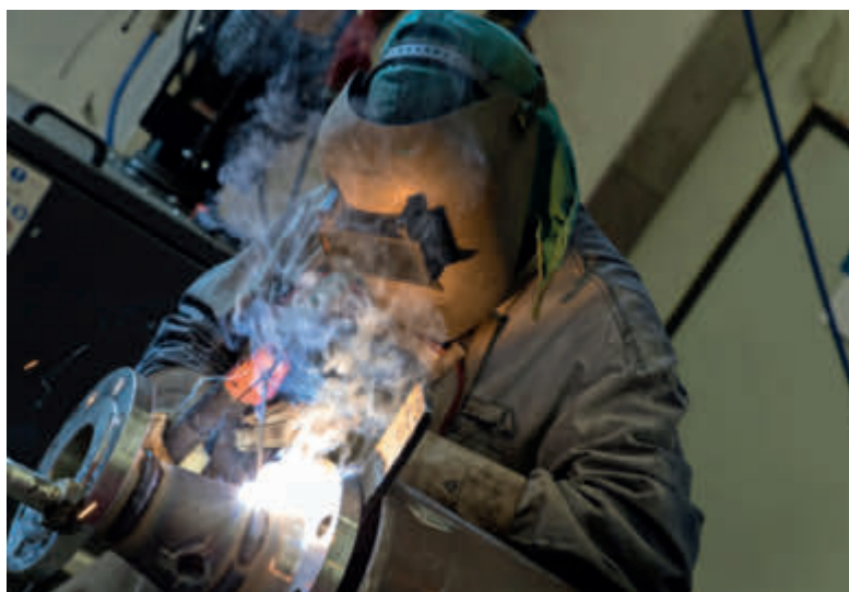
Most of the pump station components are engineered for a perfect fit under strict quality controls in the in-house metalworking shop. This simplifies on-site assembly.
