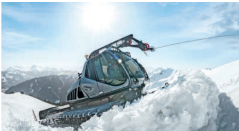
With its low-emission but high-performance Stage V engine, the new Leitwolf is an efficient machine for creating perfect slopes, also thanks to an impressive working width of 4.5 m.
