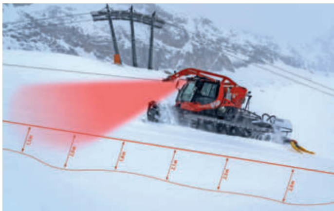
SNOWsat LiDAR provides the driver with real-time data on snow depth up to 50 m in front of and to the sides to the vehicle.
