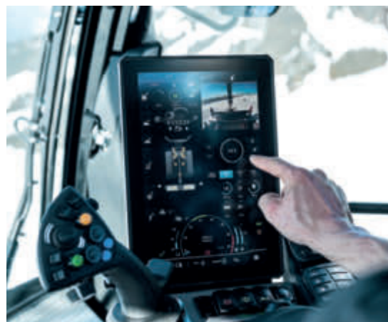
Prinoth's new user-friendly control unit in the groomer cockpit includes a joystick-in-joystick feature for simultaneous operation of all blade functions.
